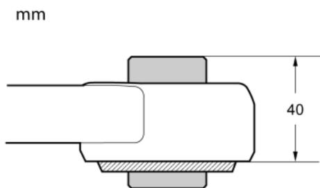
**Note! Note that the bushing's inner sleeve is longer on one side. This side must point upwards.**
