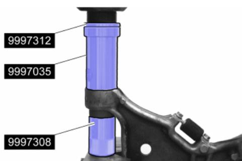
**Installing the front bushing**
